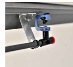
Nozzle strapped to 'L' bracket—position x
