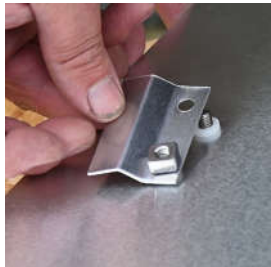
Nylon spacers on infill plate
