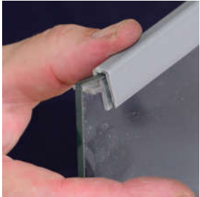
Work on handle from side edge
